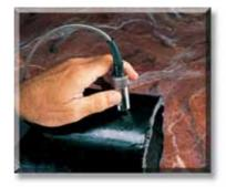
You can now forget the time-consuming removal of coatings. The TopCOAT function of the DMS 2TC helps to measure not only the thickness of the base metal, but at the same time also that of the coating layer. Moreover, you'll have other possibilities of measuring through coatings at your disposal under certain conditions, e.g. measurement within the echo sequence (Dual-Multi function). For example: Thickness measurement on parts with external corrosion.
