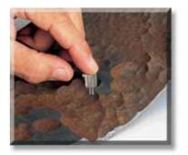
Special probes with reduced contact face enable you to measure the remaining wall thickness even at points which are normally hardly accessible: on components showing strong pitting or surface roughness due to external corrosion.
