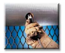
Thickness measurements on hot components are no problem with the DMS 2. We have different dual-element probes in our delivery program allowing to reliably measure components at high temperatures up to 600 °C, including coupling monitoring.
