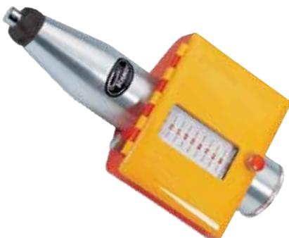
The Original Schmidt L/LR has a long tradition in roll hardness testing e.g. for hardness profiling of paper rolls. The system is easy to use and gives immediate information about the quality of the paper roll. The Original Schmidt L/LR is mostly used on the production floor. The classic rebound values "R" of the Original Schmidt LR are printed as bars on registered paper.
